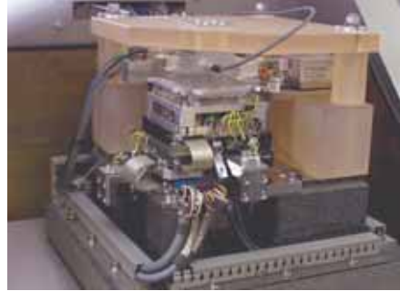
Innovation Highlight 1 Nanoscale measuring machine (0.1 nm resolution in 25 x 25 x 5 mm 3 ) © TU Ilmenau
