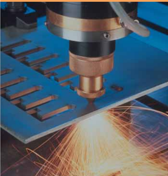
Lasers are used to cut almost everything, from organic materials to 30-mm thick steel, even diamonds. Shown here are automobile components being cut by robots with a diode-pumped solid-state laser. © ROFIN-SINAR Laser GmbH
