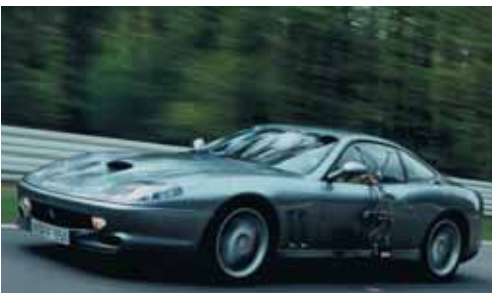
The optical sensor by Corrsys-Datron precisely measures chassis dynamics. © CORRSYS-DATRON Sensorsysteme GmbH
