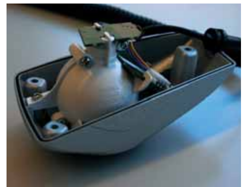
The heart of the tanning sensor is a highly precise photometric integrator made of plastic.
