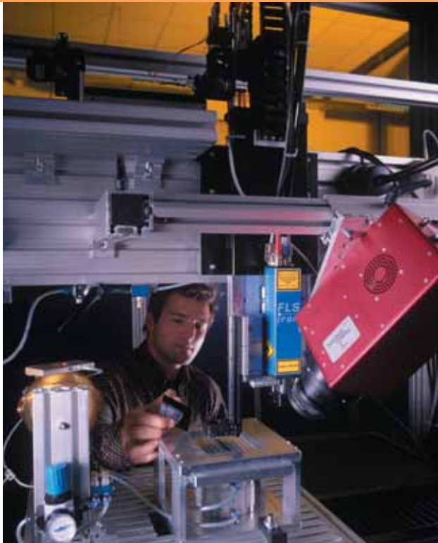
Fig. P1 In the hybrid process, laser transmission welding is combined with radiant heat welding. © BLZ/Fuchs
