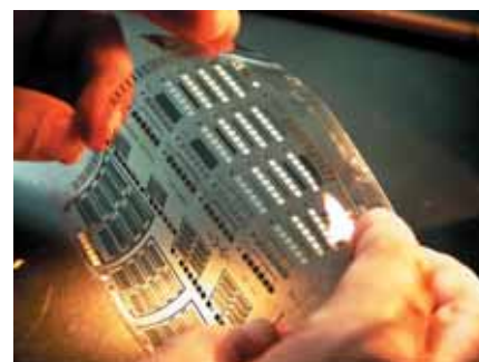
Printed polymer electronics manufactured using low-cost roll-to-roll processes © Fraunhofer Institute for Reliability and Microintegration, Munich
