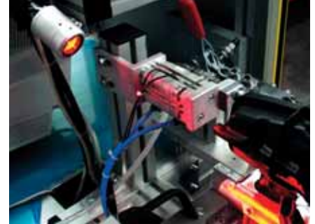
Innovation Highlight 2 Intelligent cameras and high-performance LEDs with focused beam optics in an assembly cell © GBS mbH
